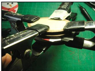
You'll need to use some flat wood and a good clamp to ensure it sticks properly. You may find a little glue will come through your joints, or even through pores in the veneer, so use a piece of plastic to stop your robin sticking where it shouldn't! Strong spring clips like those used for keeping papers together will work, but make sure they do not bruise the delicate veneers.
